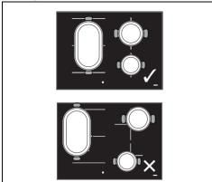
If you use a griddle, make sure that it is positioned correctly.
