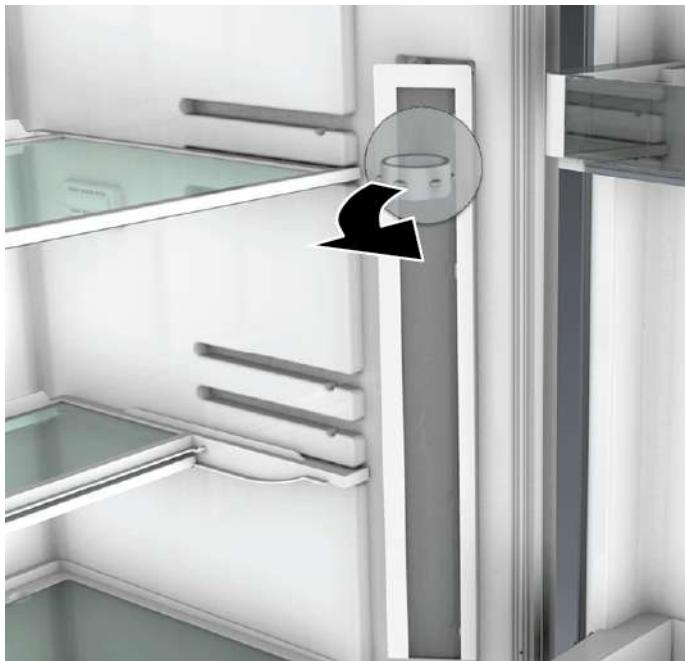
3. Disconnect electrical connection of LED side bar light.
